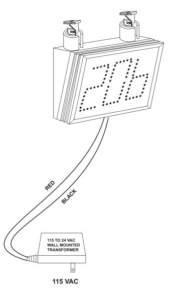
DISPLAY HANGS FROM DROP CEILING "T" BAR BRACKETS SUPPLIED
